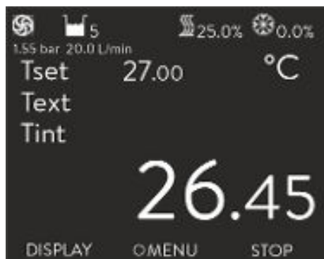
Fig. 41: Basic windows Integral XT and Integral P with through-flow control
